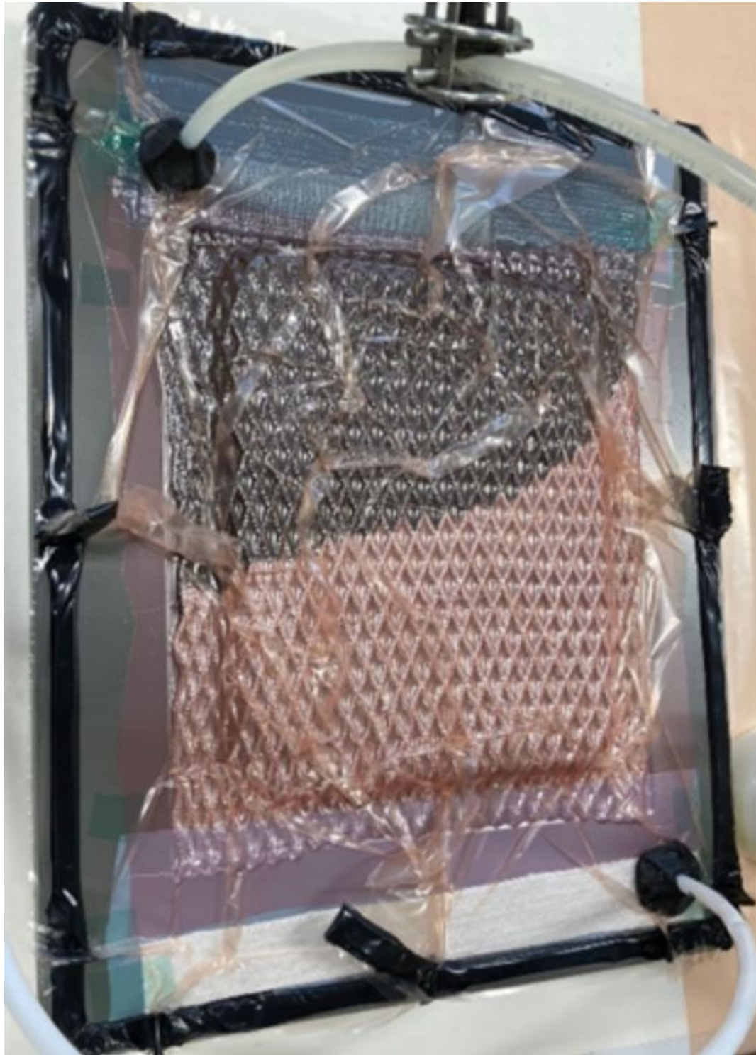
Figure 12: Left: the production of a tray with vacuum infusion; Right: the end result of the tray without hole pattern
