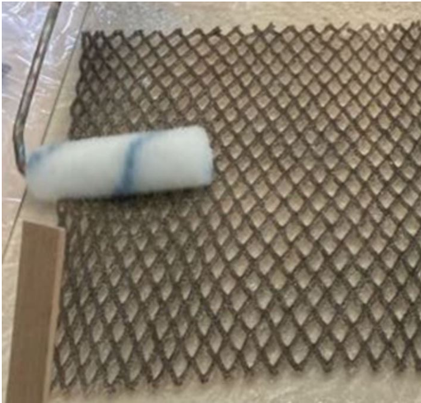
Figure 9: the hand lay-up technique: how the tray with a hole structure is produced
