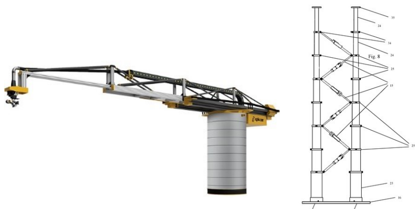
WO2018/098129 - 3-d printer on active framework - Apis Cor Engineering
